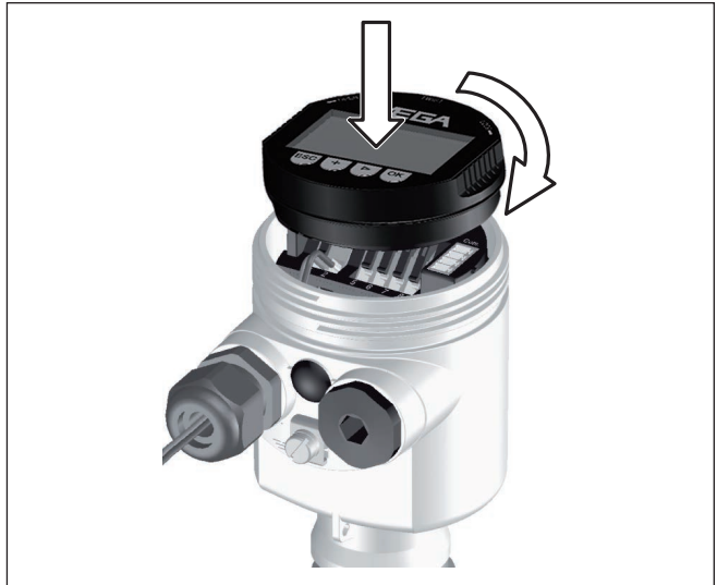
Fig. 5: Insert display and adjustment module
