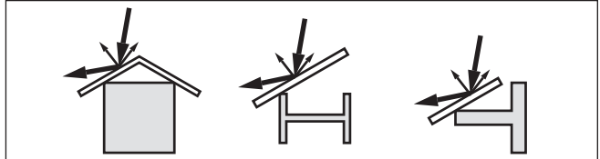
Fig. 13: Cover flat, large-area profiles with deflectors
