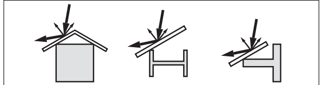
Fig. 13: Cover flat, large-area profiles with deflectors
