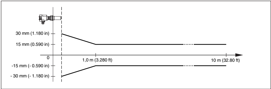
Fig. 39: Deviation VEGAPULS 61 with encapsulated antenna system and increased sensitivity
