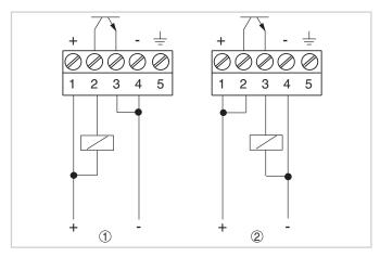
Electronics with transistor output
