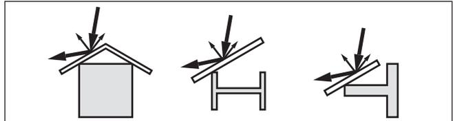
Fig. 15: Cover flat, large-area profiles with deflectors
