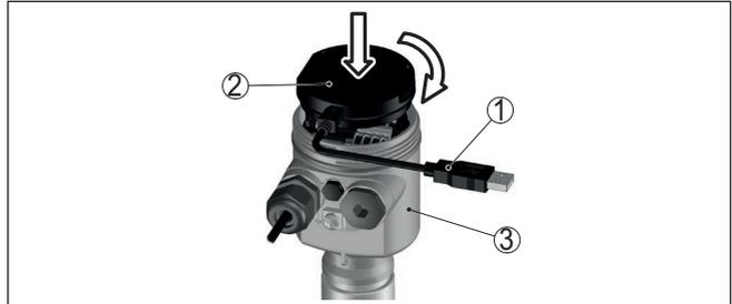
Fig. 32: Connection of the PC directly to the sensor via the interface adapter
