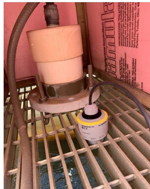
A radar level sensor and an ultrasonic transmitter are installed side-by-side to compare their performances.
