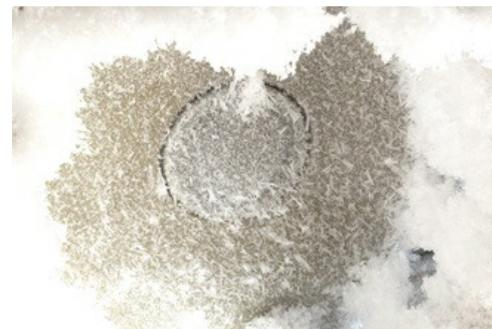
A thick layer of frost built up on the radar antenna (center circle) and on the flange.
