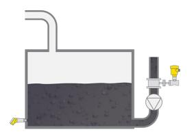
Measuring task Level and flow measurement
