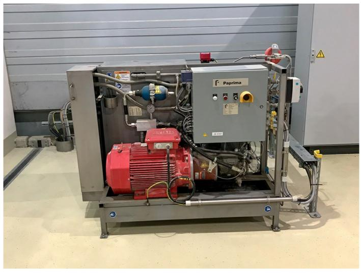
The level of the lubricating oil for the rotary lobe pumps is critical for their operation. Thanks to VEGAPULS 64, this level is now reliably
