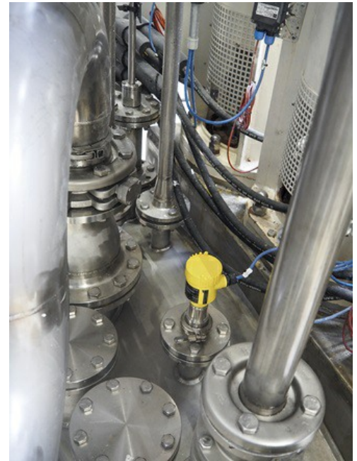
The radar level transmitter VEGAPULS 64 measures the levels in the production equipment with reliability and accuracy.
