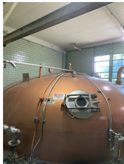
A bright yellow VEGAPULS 64 radar sensor perched atop this massive copper fermenter vessel measures level to output volume.
