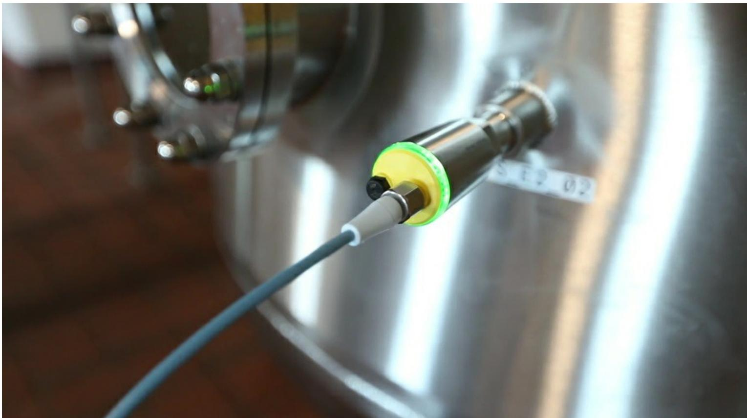
Brewery operators recognized they only needed to spray water when the foam rose too high, but they also needed to maintain a certain water level to prevent any CO<sub>2</sub> from escaping through a side vent pipe and into the cellar space. To achieve overall control of the process, they needed two point level switches – one that could switch the spray ball on when it sensed the foam was too high and another that would switch the spray ball on if the water level dropped too low.
