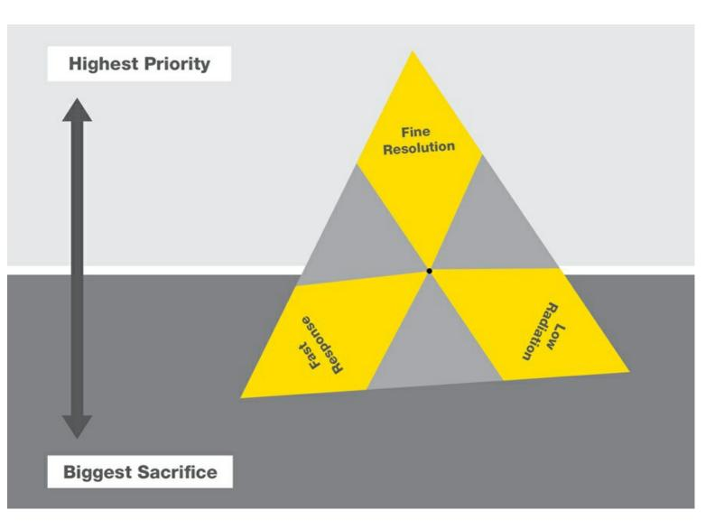
Source activity, or radioactivity, has a direct relationship with resolution and response time. With a higher activity, resolution improves and response time decreases. The ratio at which this happens is roughly 4:2, meaning the source activity needs to be quadrupled to double the resolution or half the response time. This somewhat unfavorable ratio typically leaves the user making some tough decisions if they want to minimize the amount of radioactivity at the source.
