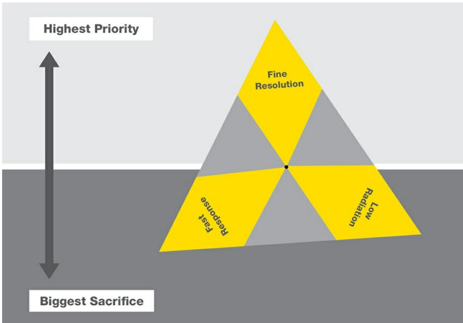
Source activity, or radioactivity, has a direct relationship with resolution and response time. With a higher activity, resolution improves and response time decreases. The ratio at which this happens is roughly 4:2, meaning the source activity needs to be quadrupled to double the resolution or half the response time. This somewhat unfavorable ratio typically leaves the user making some tough decisions if they want to minimize the amount of radioactivity at the source.
