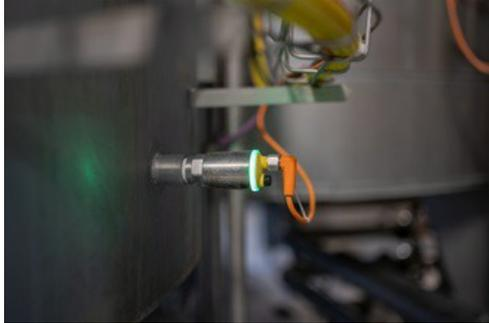
The point level plays a crucial role at several points in the brewing process – at Alpirsbacher, for example, the VEGAPOINT level switch is used in the grist mill. This is where the malt is crushed before brewing. This point level sensor immediately detects when a certain value is reached and reports this. It prevents the mill from overflowing or running idle without malt, which can waste energy and lead to damage in the long term.
