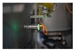
The point level plays a crucial role at several points in the brewing process – at Alpirsbacher, for example, the VEGAPOINT level switch is used in the grist mill. This is where the malt is crushed before brewing. This point level sensor immediately detects when a certain value is reached and reports this. It prevents the mill from overflowing or running idle without malt, which can waste energy and lead to damage in the long term.
