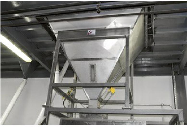
The level in the pellet container is reliably measured and can be kept constant.
