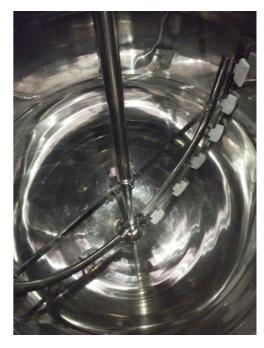
During operation, continually rotating scrapers ensure the vessel heating jacket is free of buildup. The focused beam of VEGAPULS 64 radar level sensor ignores these scrapers easily.
