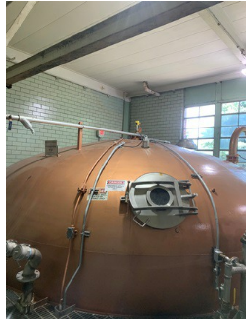
A bright yellow VEGAPULS 64 radar sensor perched atop this massive copper fermenter vessel measures level to output volume.
