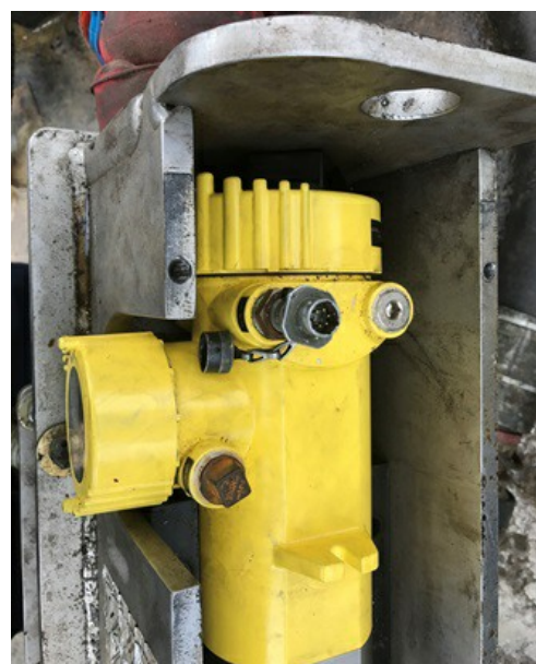
MiniTrac 32 is particularly suitable for applications with extreme vibration
