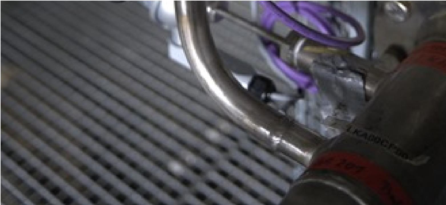
VEGABAR 83 pressure transmitters are in use.
