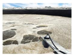
Foam, deposits and heat greatly affected the previously used level sensors and led to inaccurate measured values. The compact VEGAPULS C 21, which is based on 80-GHz technology, has a fixed cable connection so that it can withstand flooding. From the very beginning it has delivered reliable measurement data.
