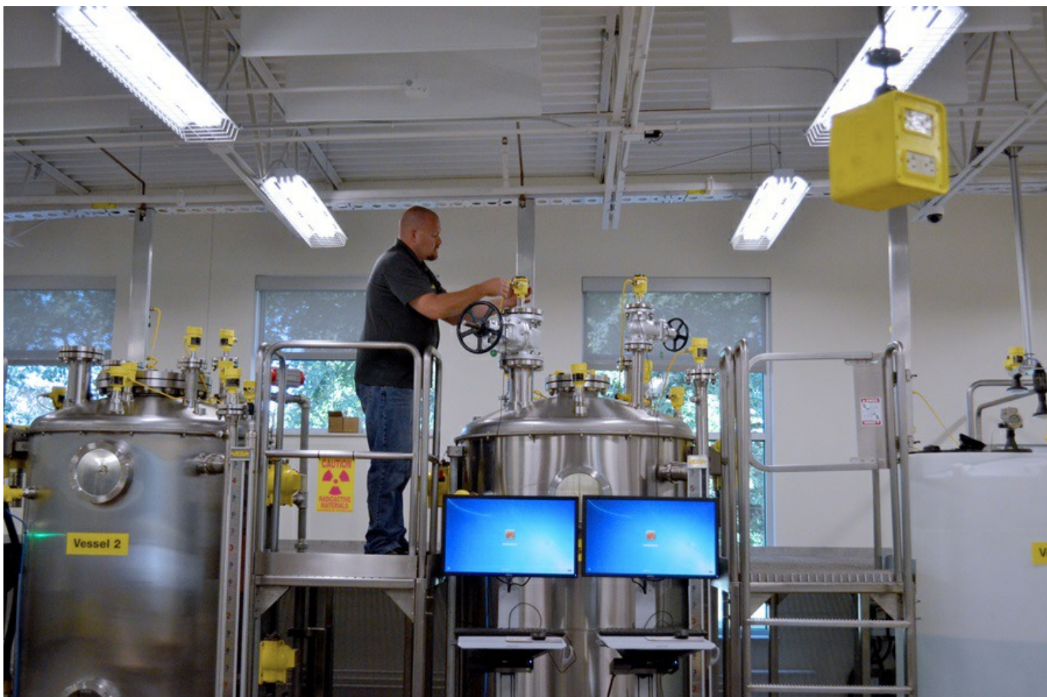
VEGA Americas Field Service Technician Dan Nartker readies a pair of VEGAPULS 64 sensors for testing with gate valves.
