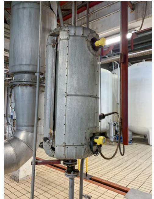
Pressure sensors of type VEGABAR 82 monitor the concentration of tartaric acid, an important component of grappa.
