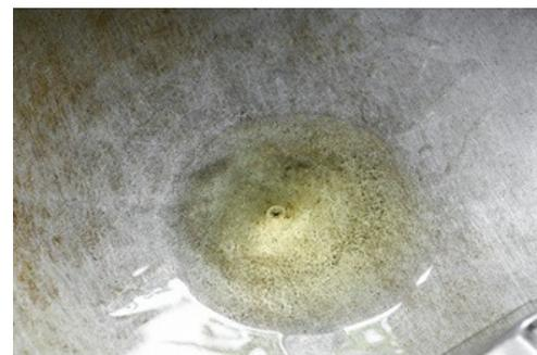
Oil on the tank floor. At low levels, it is very difficult to measure oils or other liquids accurately.
