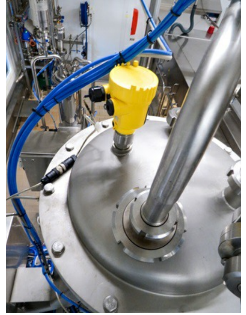
VEGA sensors control the level to keep the yoghurt filling process running smoothly.
