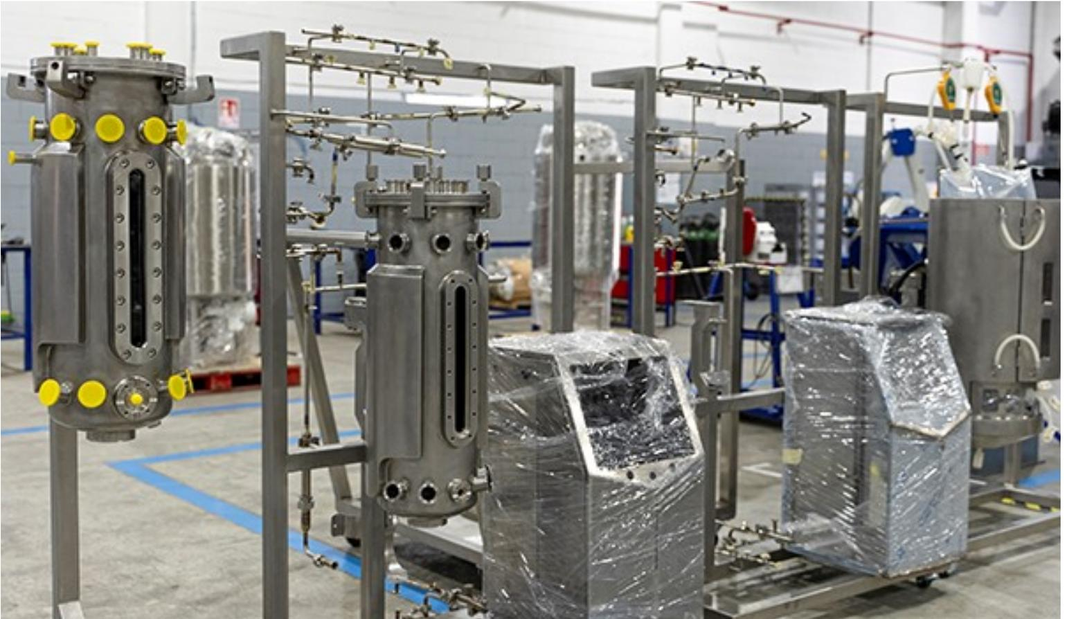
A wide variety of VEGA sensors are installed in the processing systems. These deliver their analogue and digital 4 ... 20 mA signals to TECNIC's own eSCADA software. Based on the AVEVA platform, the software manages the control parameters and ensures that the recipes are adhered to in compliance with GAMP5 and CFR21. "We set up and commission all the sensors ourselves. But if we do need help, we can always rely on VEGA's technical support," adds Estany.
